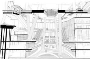
The large steel beam , inclined columns and facades Source: www.greatnewplaces.com
